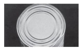
Double seam not severely damaged .
